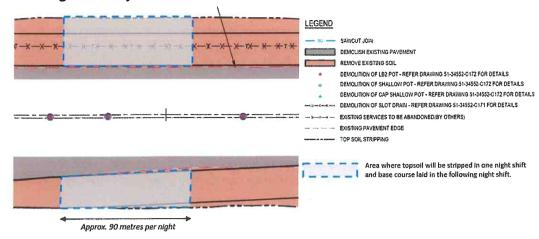
Striping of topsoil soem night of base course being laid. This will be undertaken in lengths of 90m--150m per night. Following each night shift the finished compacted basecourse surface area coated with an emulsion to prevent any sediment runoff.
