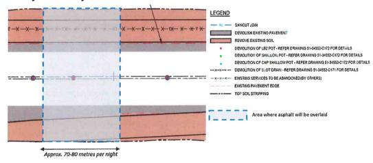
Asphalt will be laid across the full width of the taxiway, in lengths of 70-80m per night working from the north to the south.
