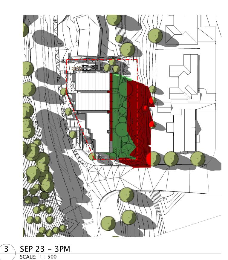
HATCH INDICATES HEIGHT AND SUNLIGHT RECESSION PLANE BREACH SHADOW INDICATES BASELINE MODEL SHADOW
