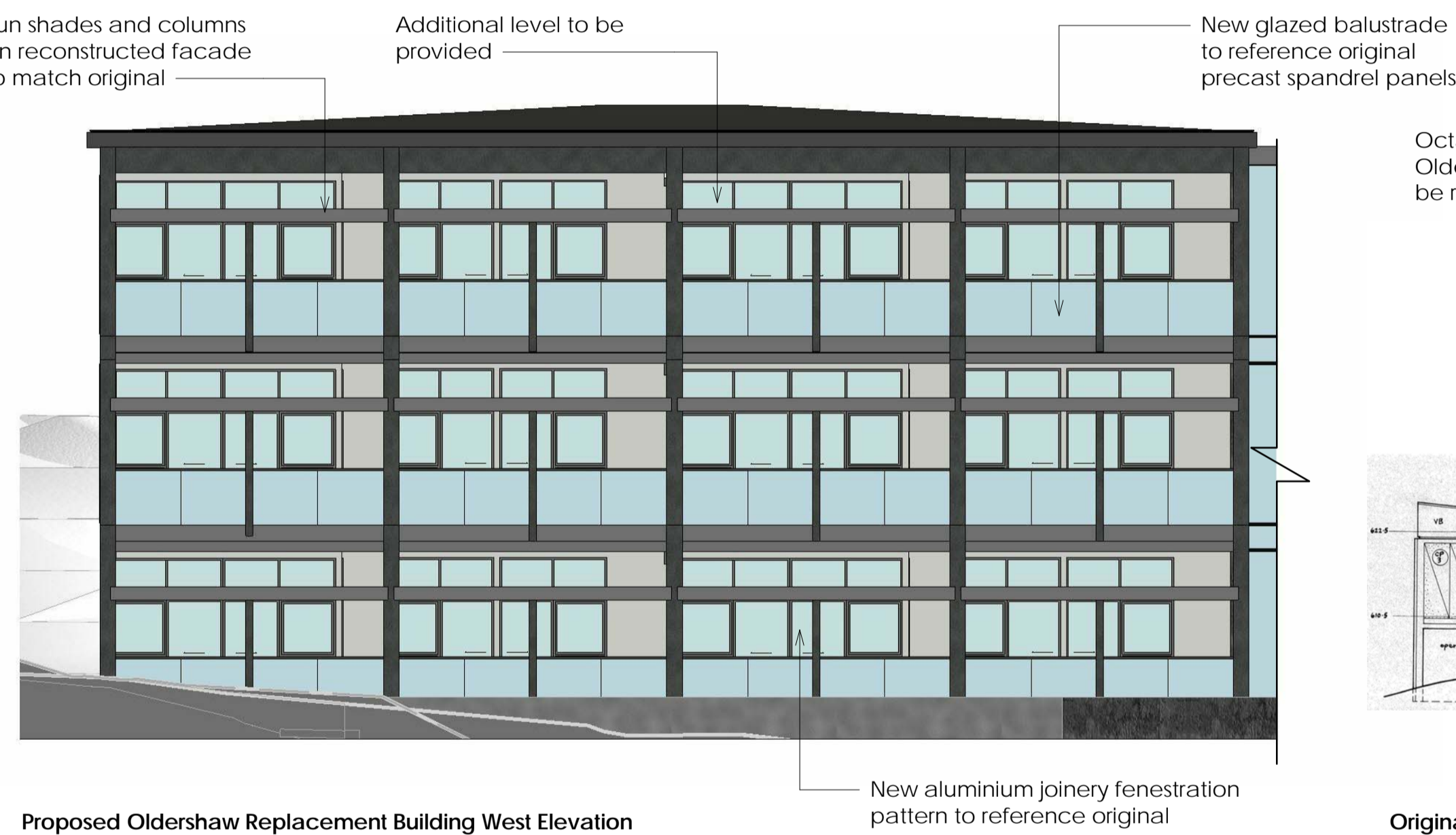
Proposed Oldershaw Replacement Building West Elevation
