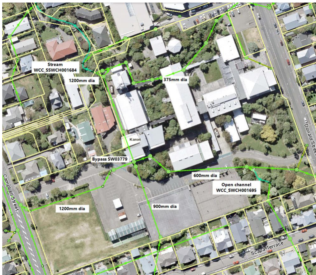
Figure 2 Existing Public Stormwater Network
