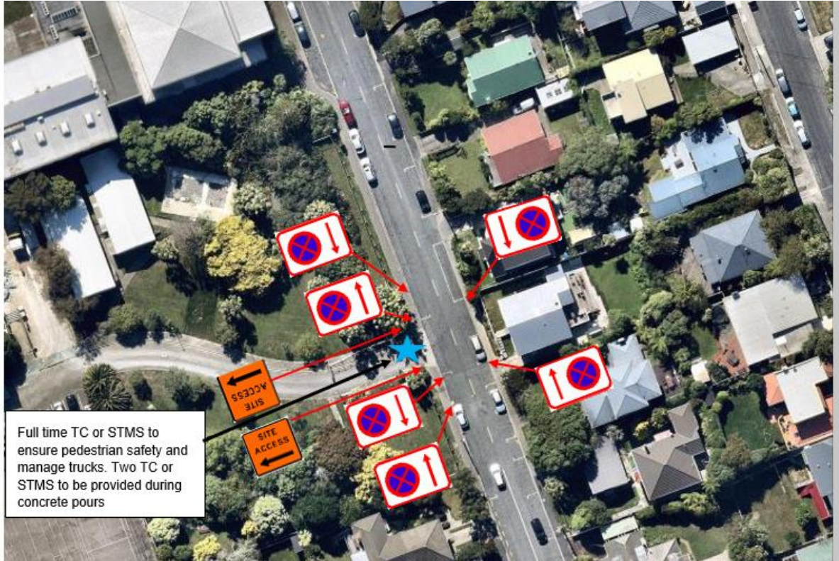
Figure 6: Traffic Controls / Parking restrictions at Donald Street access point
