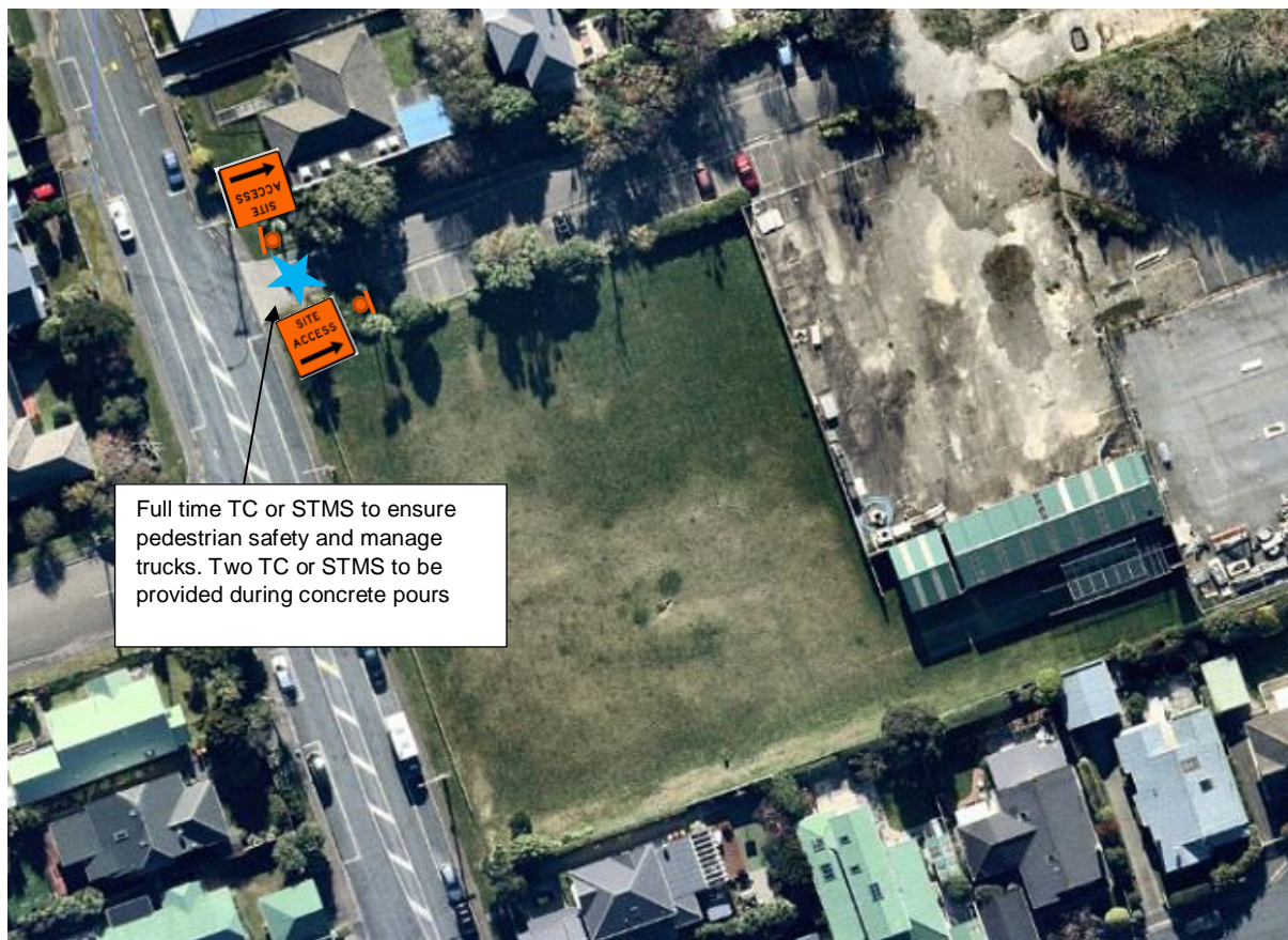
Figure 8: Traffic Controls at Campbell Street access point
