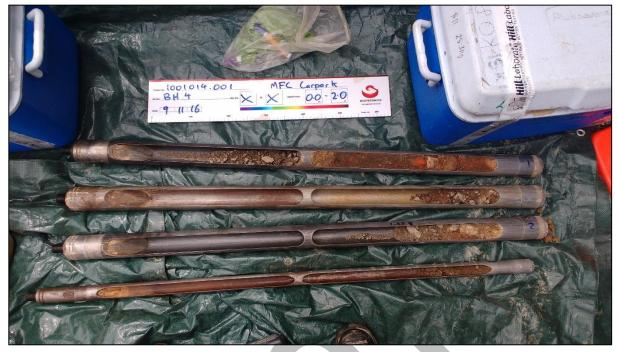
Photograph 6: Recovered core from BH4. Photo taken on 9 November 2016. Photo sourced from Geotechnics Limited.
