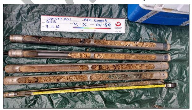
Photograph 5: Recovered core from BH5. Black gravels/slag can be observed at 0.3 m. Photo taken on 9 November 2016. Photo sourced from Geotechnics Limited.
