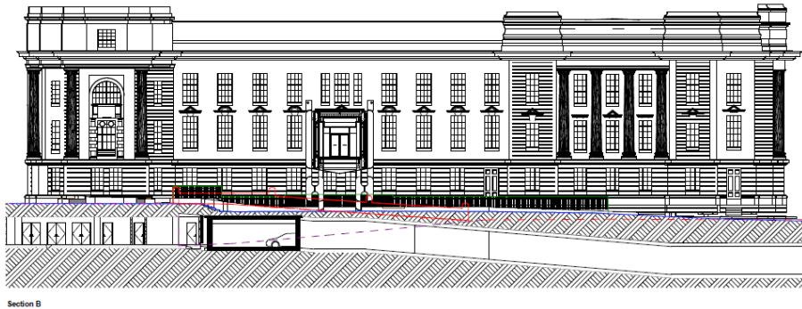
Figure 5 Studio Pacific Architecture section showing the proposed plaza ground level west of the “slot”. The proposed railings are shown.
