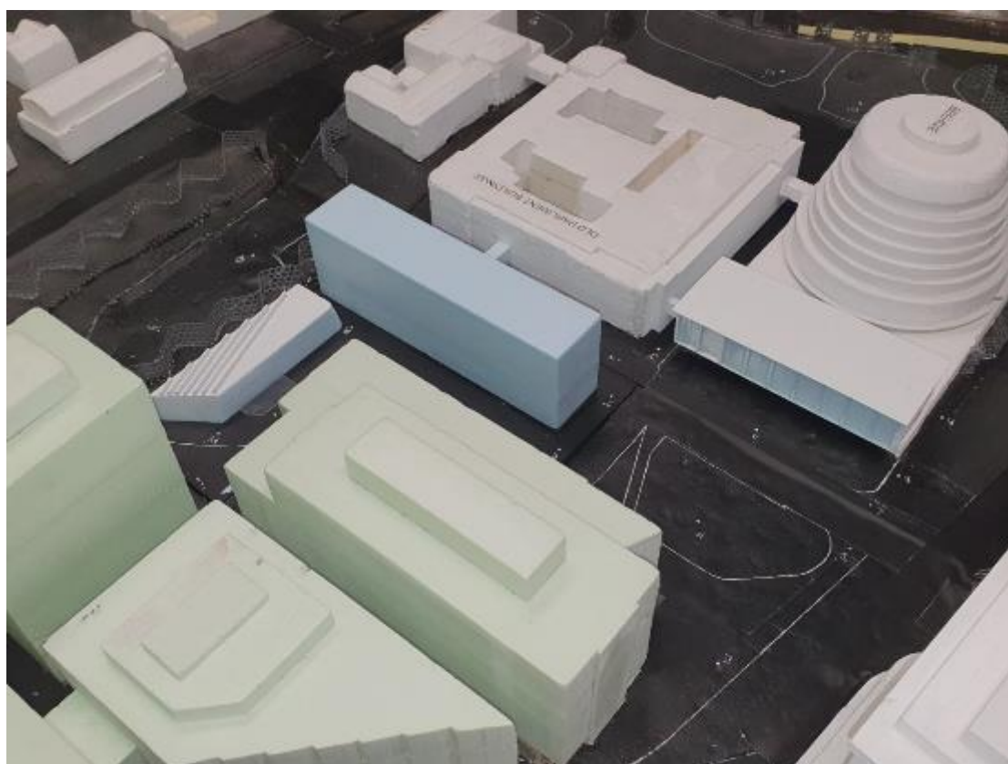
Figure 2(b): Wind tunnel model of the development proposal that was wind tunnel tested, viewed from the southeast.
