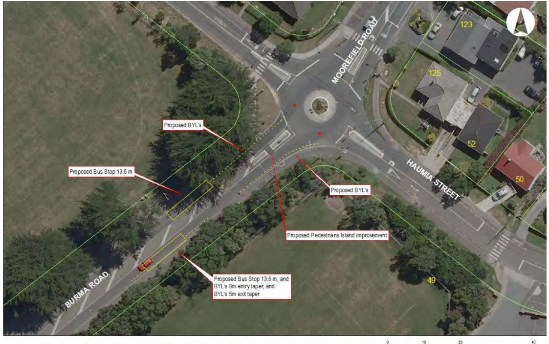
Burma Rd Johnsonville TR (71-14) Proposed 2 Bus Stops & No stopping at all times
