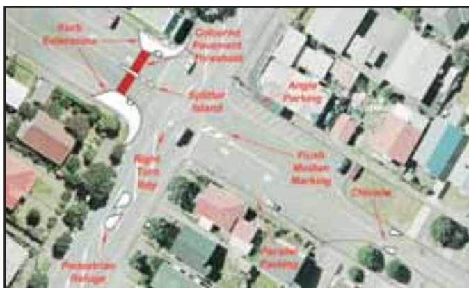
This drawing shows examples of traffic features listed in the draft implementation plan on pages 6 and 7.
