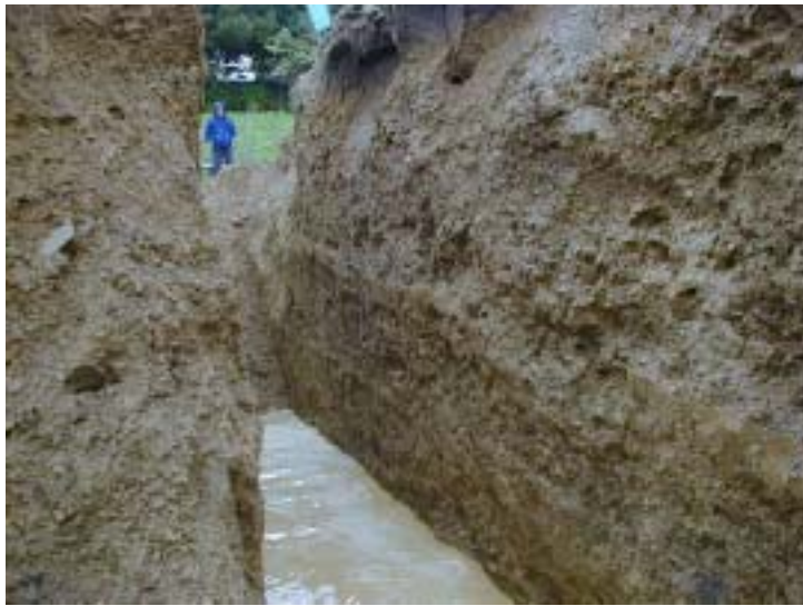
Figure 5 Fault investigation trench at former Thorndon Bowling Club site Goring Street. Photos: N.D. Perrin, 19 July 2001, courtesy of Ian R Brown Associates Ltd.
