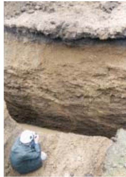
Figure 6 Fault location in trench. Photos: N.D. Perrin, 19 July 2001, courtesy of Ian R Brown Associates Ltd.
