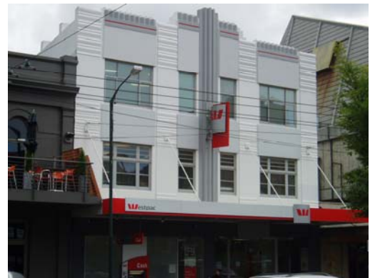
Good example of a corporate logo/sign that is in scale and compatible with the heritage character of the building
