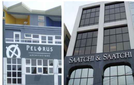
Signs composed of individual letters and not placed on any backing panel are less dominating and integrate better with the building
