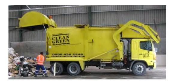
The potential for the recovery of materials from waste transported by front-loaders is limited. The waste load is compacted by the truck, and the loads tend to be large and heterogeneous. This restricts significantly the potential for manually separating recoverable materials when the load is discharged on a tipping floor. There are usually not significant quantities of easily-separable materials other than cardboard packaging in front-loader refuse.
