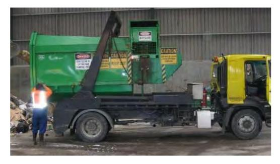
Typical gantry truck loads weigh from 0.5-3 tonnes. As most refuse transported in gantry bins is not compacted, there is often opportunity for manually recovering materials from gantry bins when discharged onto a tipping floor. Gantry bins often contain significant quantities of recoverable materials, such as timber and packaging, and these materials as well as reusable items can often be recovered intact from loads.
