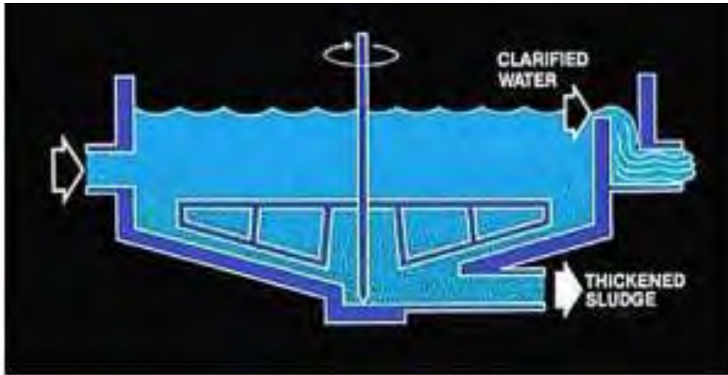
Figure 1: Schematic of a Static Gravity Thickener
