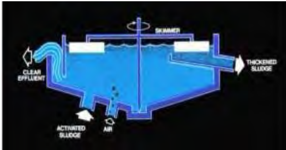
Figure 3: Schematic of a Dissolved Air Flotation Apparatus
