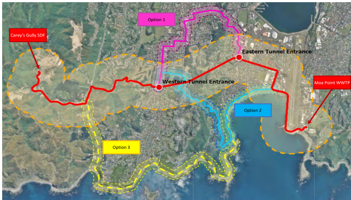
Figure 5-2: Sludge transfer pipeline options
