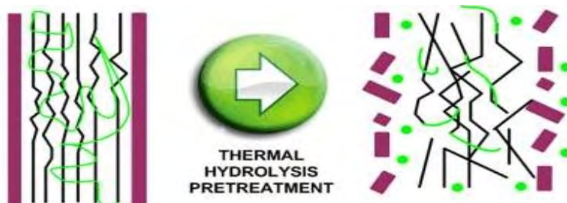
Figure 4-7: Schematic of Cell Wall Breakdown during THP Pre-treatment.
